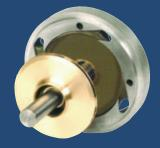
L50 Series inducer style pumps are designed specifically for applications where the net positive suction head available at the pump inlet is limited, such as in boiler feed water deaerator service.
